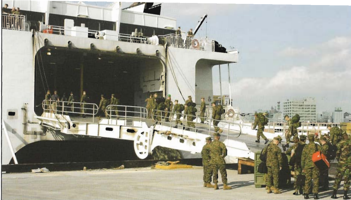
Figure 3: As part of a redesign, a large folding ramp was fitted to the stern of the WestPac Express , to enable loading and discharge of vehicles and cargo.
